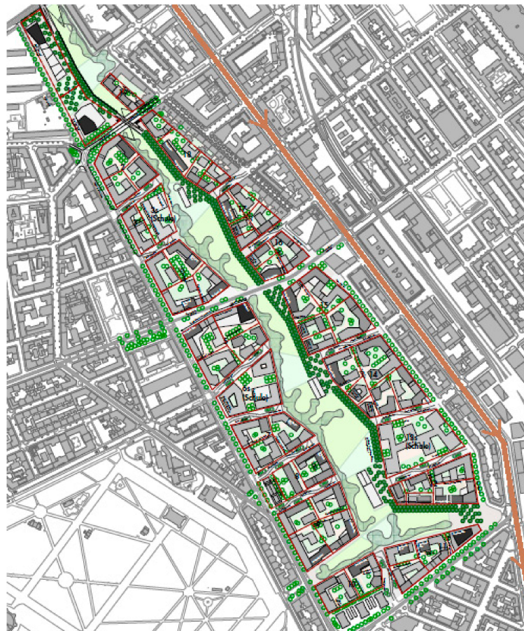
Figure 1. Overview over the intended building positions and types of use at “Nordwestbahnhof” development area, adapted with permission from [31] OEBB (internal document): Vienna, Austria, 2019, including the main sewer at the right (in brown), arrows indicate flow direction.
