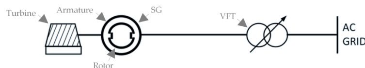
Figure 3. Connection through a VFT.
