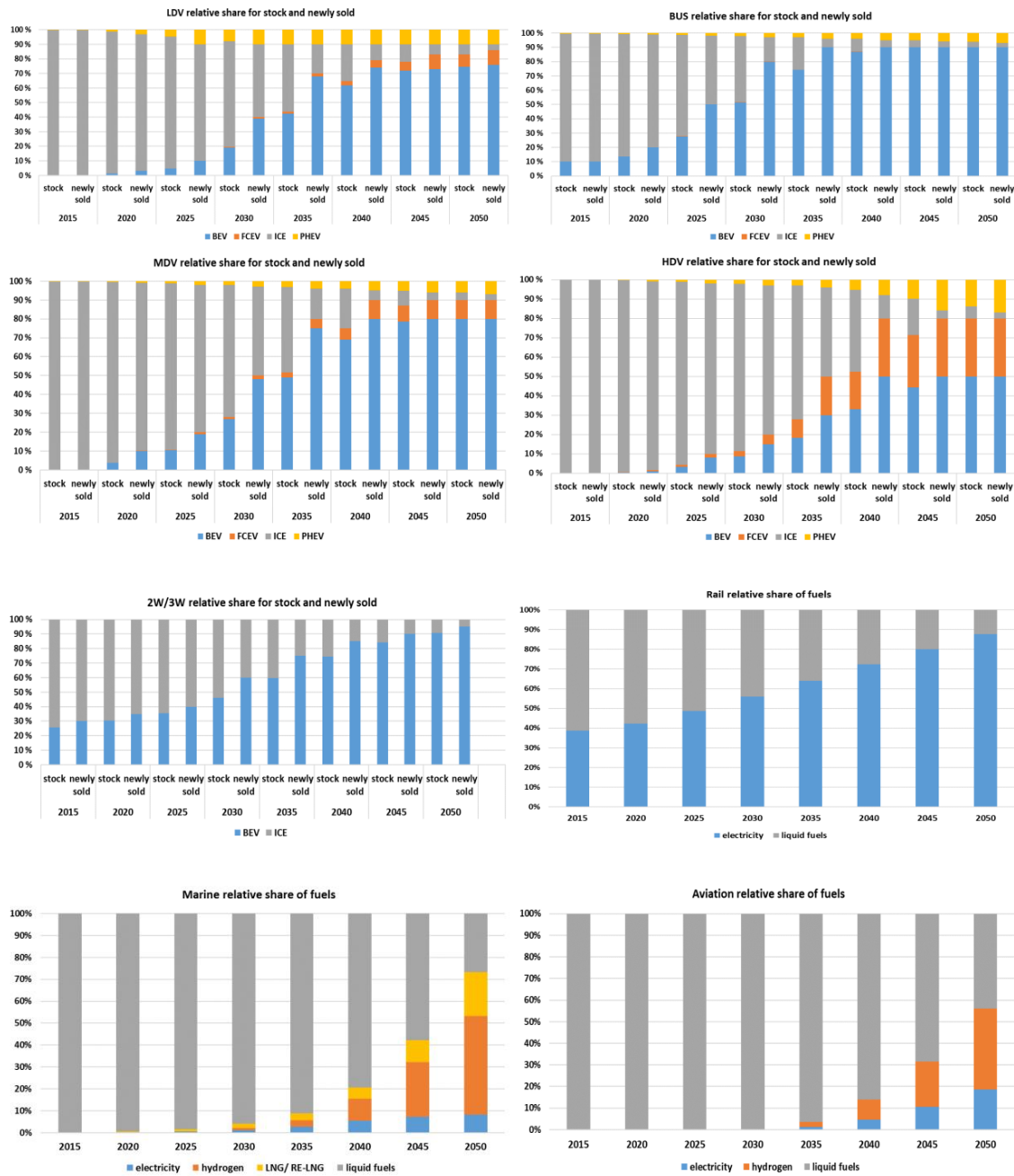
Figure 12. Vehicle types and fuel shares of LDV (top left), BUS (top right), MDV (center top left), HDV (center top right), 2W/3W (center bottom left), rail (center bottom right), marine (bottom left), and aviation (bottom right) for the years 2015 to 2050.
