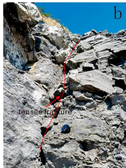
(b) Tensile fractures are developed in the interlayer formed by mudstone and the middle-thick limestone of the Shiniulan Fm., which are filled with large amounts of calcite.
