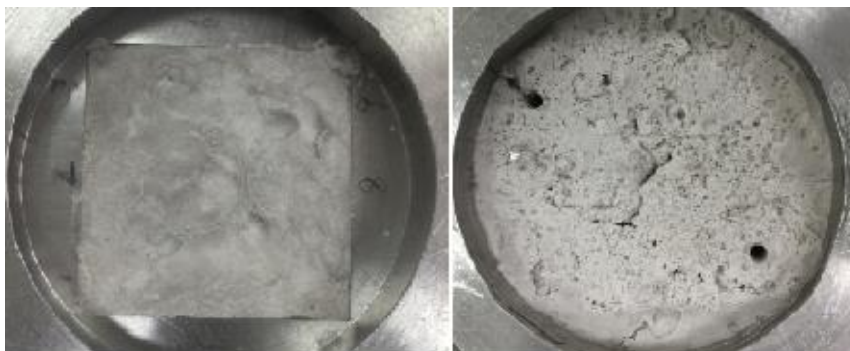
Figure 10. Sediment morphology before and after hydrate dissociation for run 2.
