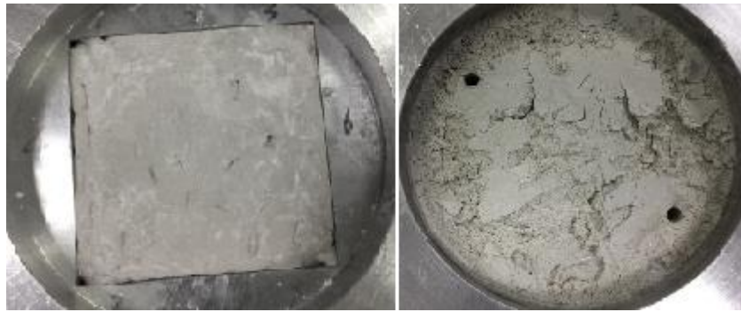
Figure 11. Sediment morphology before and after hydrate dissociation for run 3.
