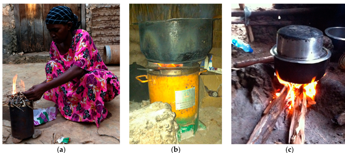
Figure 2. (a) Lighting fuel in a canister outside; (b) cooking with gasifier; and (c) cooking with three-stone open fire.
