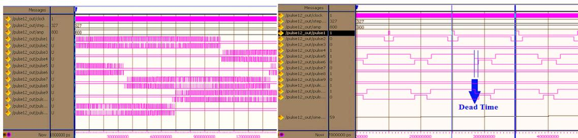
Figure 15. ModelSim simulation results; 12-pulses ( $S_{1u}$ – $S_{4w}$ ) of proposed MLI SVM for  $f_s = 10$  kHz, dead time = 6  $\mu$ s.
