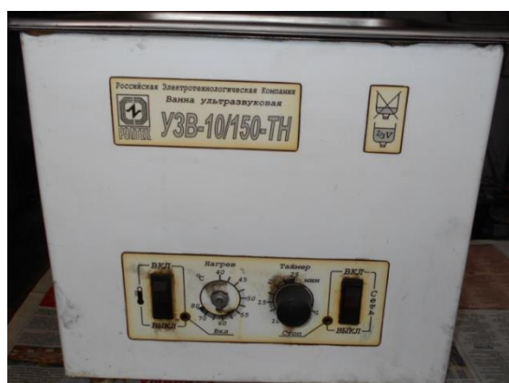
Figure 4. Ultrasonic bath used for preparing mixtures of petroleum diesel fuel with carbon nanotubes (CNTs).
