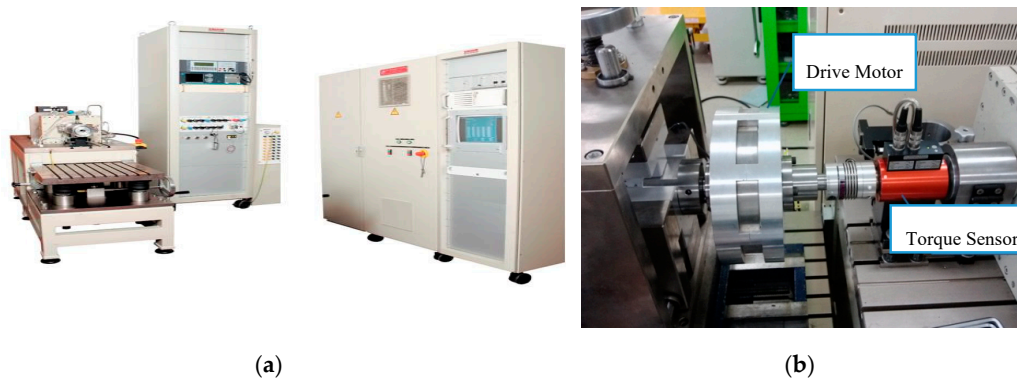
Figure 9. Inductor test equipment and test device configuration: (a) Induction motor test equipment, (b) test device configuration.
