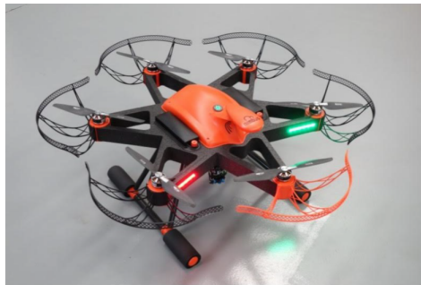
Figure 5. The adopted exacopter, equipped with an optical camera (Lumix DMC-G1) and a thermal camera (FLIR A65).
