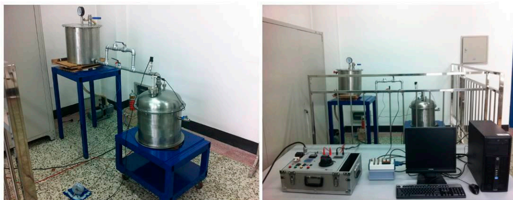
Figure 6. Discharge-fault simulation system and operating platform.
