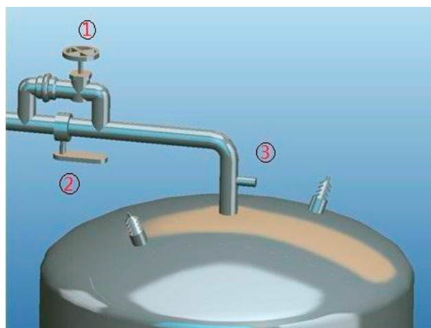
Figure 3. Schematic of valve setting in oil-pressure-monitoring test chamber.
