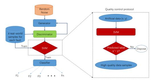
**Figure 3.** Proposed framework for AHU fault diagnosis based on Wasserstein GAN (WGAN) and support vector machine (SVM).
