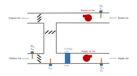
**Figure 1.** The general structure of the Air handling unit (AHU) used in ASHRAE project No. RP-1312 with critical features marked.
