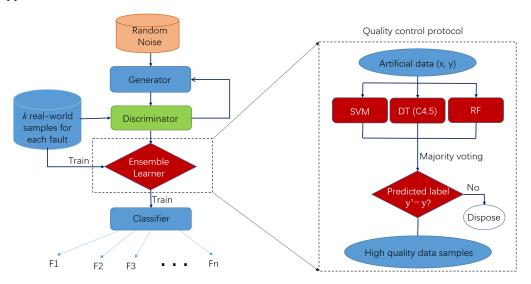
**Figure 4.** An extension of the proposed framework combining WGAN with an ensemble learning structure.
