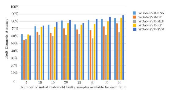
**Figure 5.** Classification/diagnosis results comparison between various classifiers using WGAN-SVM to generate artificial faulty training samples.
