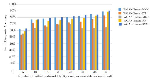
**Figure 6.** Classification/diagnosis results comparison between various classifiers using WGAN-ensemble to generate artificial faulty training samples.
