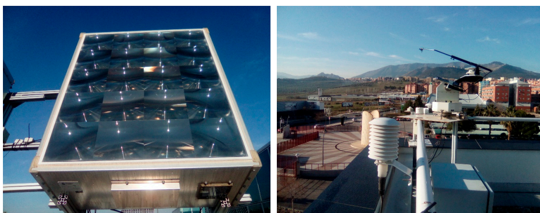
Figure 6. Experimental set-up used to conduct this study at the Centro de Estudios Avanzados en Energía y Medio Ambiente at the University of Jaén. (left) HCPV module; (right) atmospheric station.
