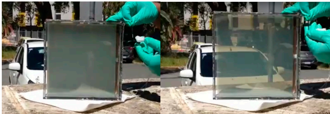
Figure 5. Transparency-controlled, self-powering PDLC-integrated “smart” solar window demonstration at Edith Cowan University (ECU) in October, 2014. A 200 mm × 200 mm hybrid concentrator-type solar window used four parallel-connected edge-mounted CuInSe 2 modules of size 198 mm × 25 mm, the electric output of which was sufficient to control the embedded PDLC layer transparency within a broad transparency range [108].
