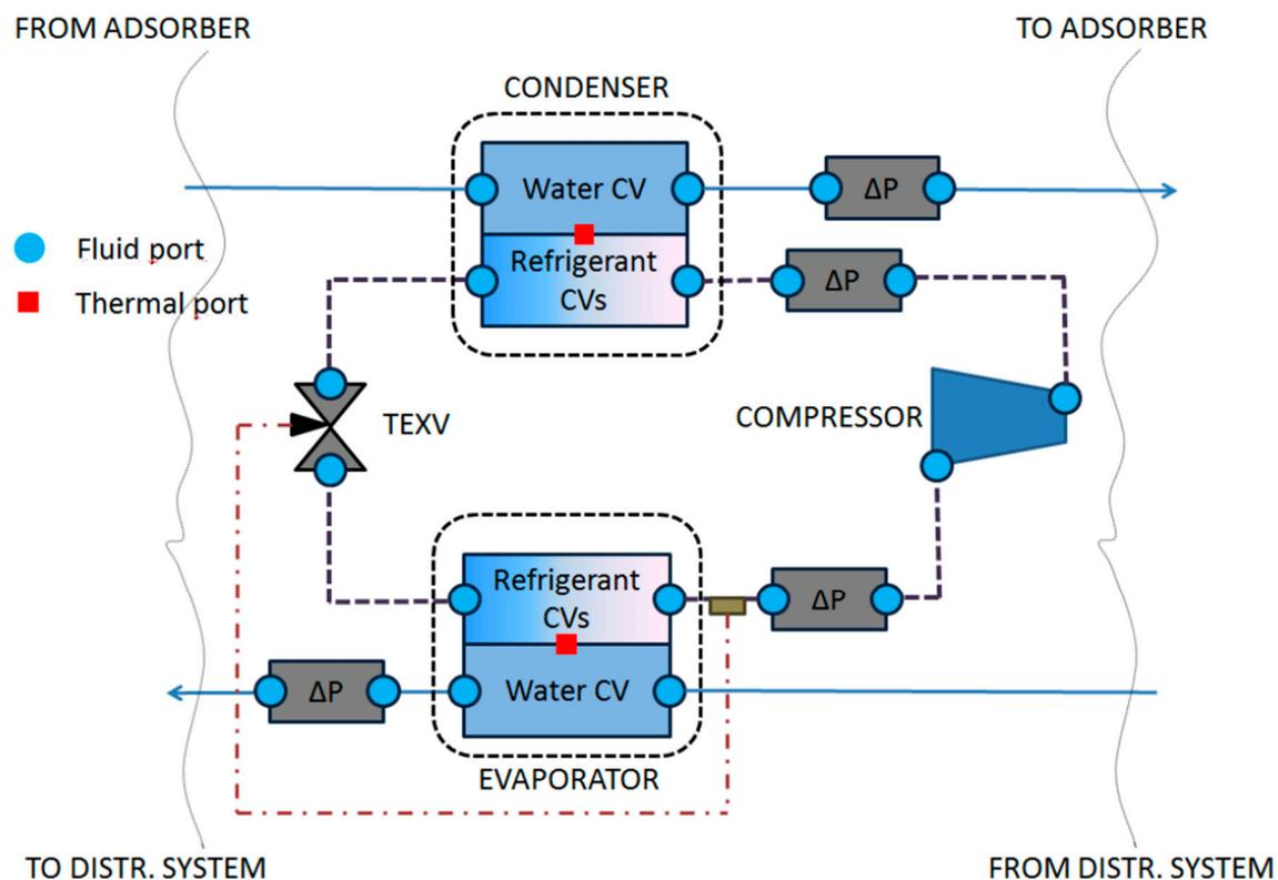
Figure 6. Compression chiller model layout representing the Dymola implementation.
