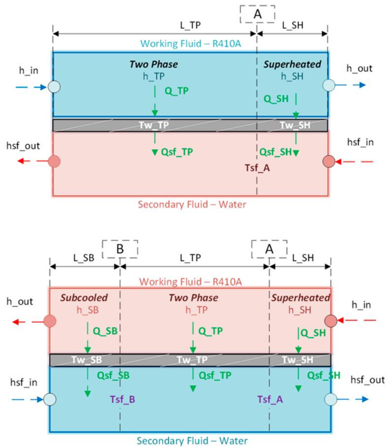
Figure 5. CV formulation for the evaporator (up) and the condenser (bottom) heat exchanger models.
