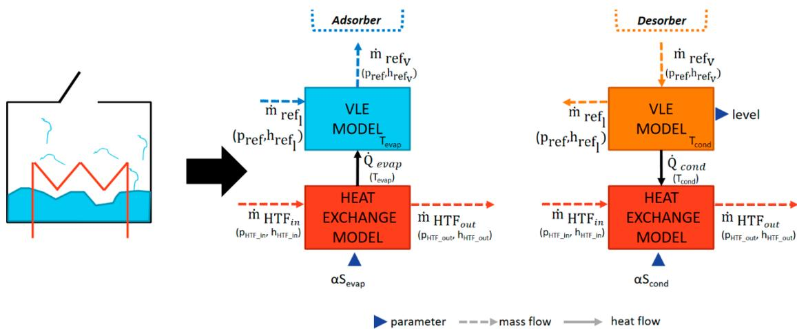
**Figure 3.** Schematics of the adsorber (left) and its implementation, with input and output variables and energy flows for the adsorber during adsorption (middle) and desorption (right).
