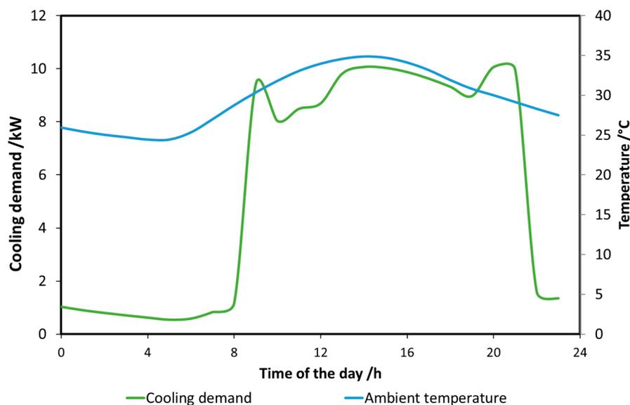
**Figure 11.** Boundary conditions for the dynamic simulation of the hybrid system - temperature and cooling demands for a reference day in Aglantzia (CY).
