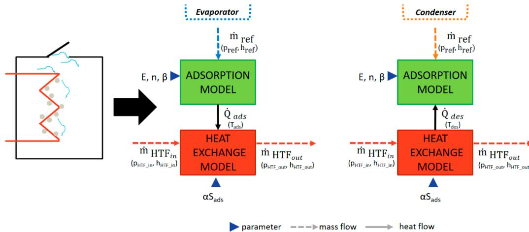
**Figure 4.** Representation of the evaporator/condenser (left) and its implementation, with input and output variables and energy flows for the evaporator (middle) and condenser (right).
