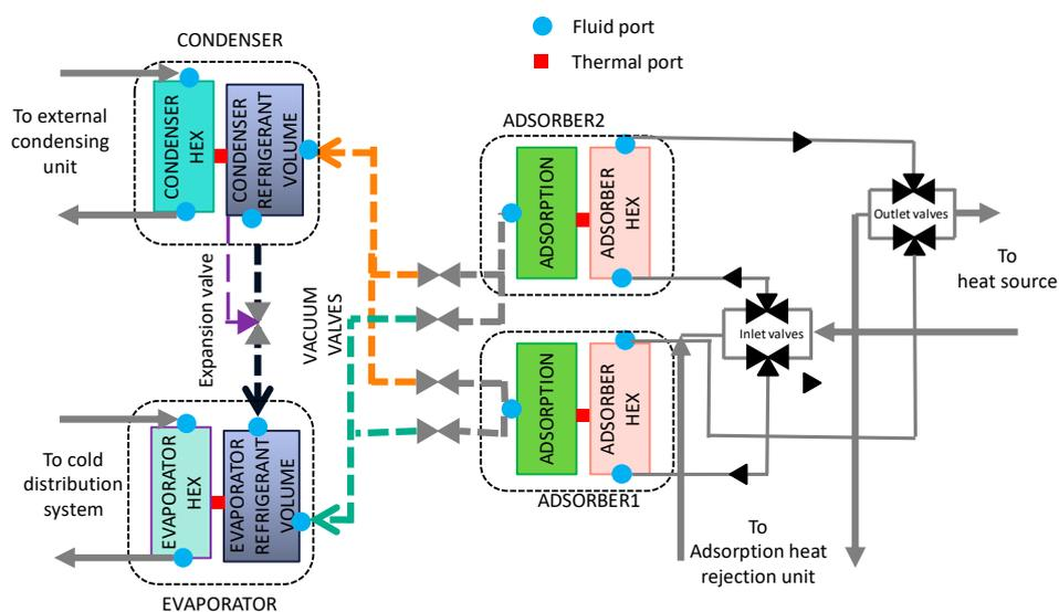
**Figure 2.** Layout of the model of the adsorption module with the indication of fluid ports and thermal ports as in the model implementation in Dymola.
