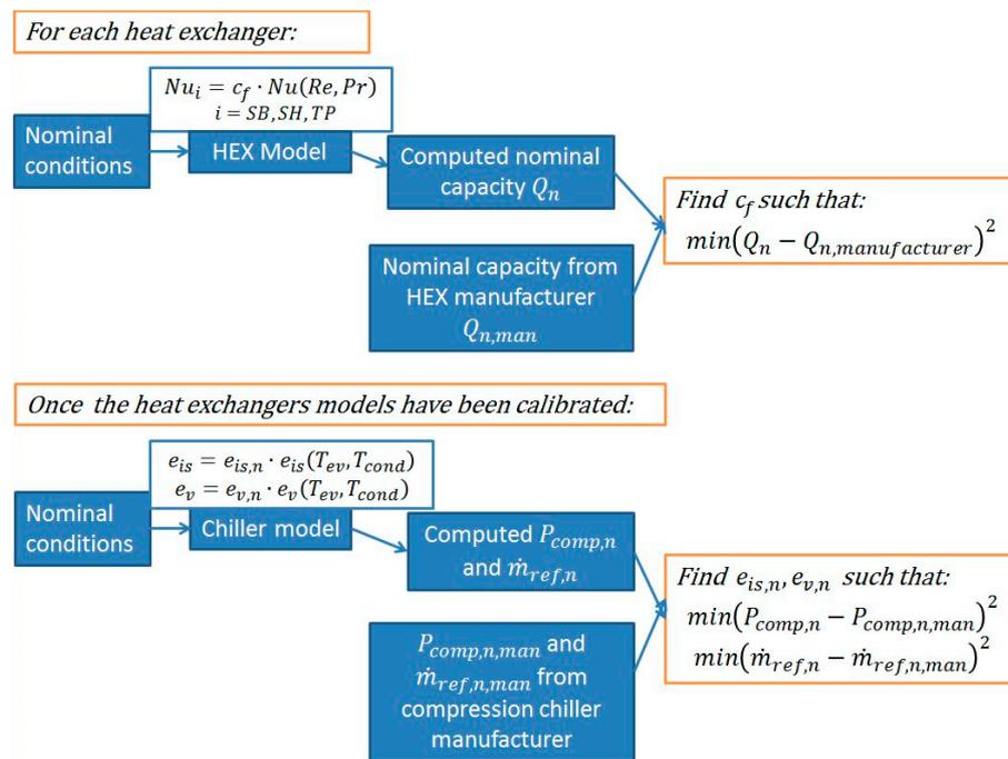
Figure 8. Representation of the compression chiller model calibration procedure.
