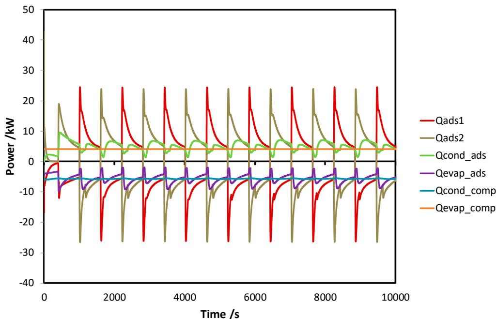
**Figure 13.** Thermal powers in the components of the sorption module and the vapour compression chiller for the reference conditions.
