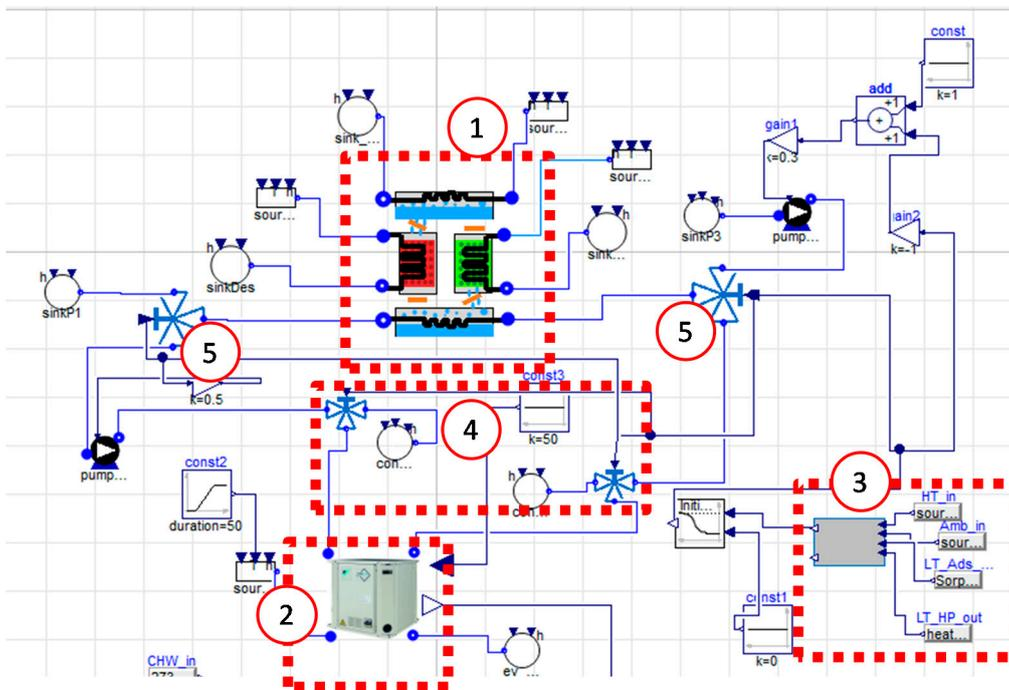
**Figure 10.** Dymola layout of the hybrid integrated model. 1: sorption module; 2: compression chiller; 3: control unit; 4: 3-way valve for switching between heating and cooling mode of the compression chiller; 5: 3-way valves to switch between the hydraulic connections of the units and the direct connection of the compression chiller to the heat rejection (medium temperature) circuit.
