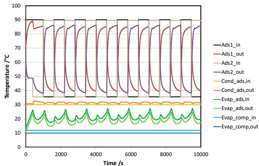
**Figure 12.** Temperatures in the circuits of the sorption module and heat pump for the reference conditions. The outlet of the evaporator of the adsorption unit (light green) also represents the inlet of the condenser in the vapour compression chiller; the inlet of the of the evaporator of the adsorption unit (dark green) also represents the outlet of the condenser in the vapour compression chiller.
