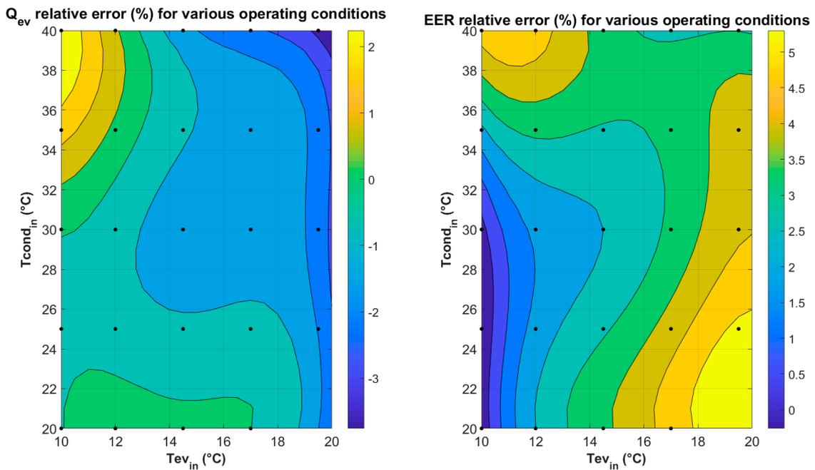
**Figure 9.** Compression chiller validation results in terms of relative errors (%) for the evaporator capacity and the EER under various inlet water temperatures.
