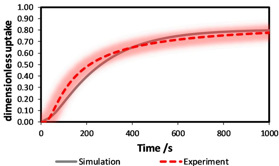
Figure 7. Validation of the model for the adsorber. The red area represents experimental error.
