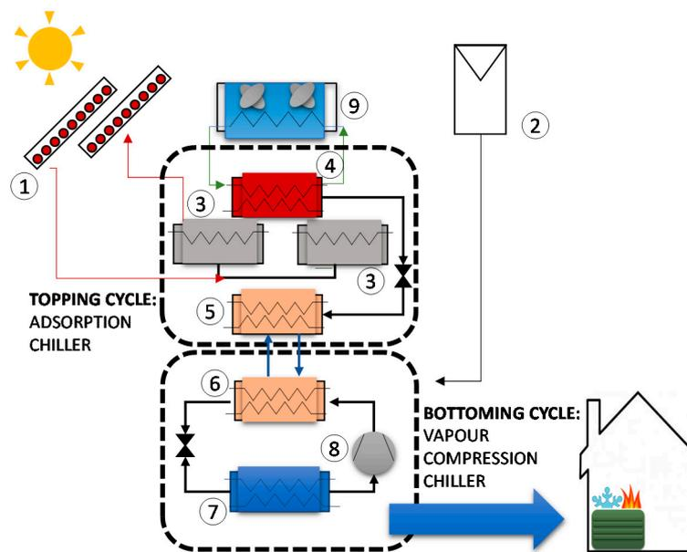
**Figure 1.** The hybrid system proposed: (1) solar thermal collectors field. (2) photovoltaic panels. (3) adsorbers of the adsorption chiller. (4) adsorption chiller condenser. (5) adsorption chiller evaporator. (6) vapour compression chiller condenser. (7) vapour compression chiller evaporator. (8) compressor. (9) dry cooler for heat rejection to the ambient.
