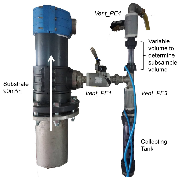
Figure 3. Physical construction of the three valves Vent_PE1 , Vent_PE3 and Vent_PE3 to define subsample volume according to the enclosed air volume, V_{enclosed} .
