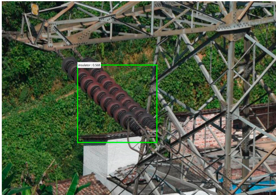
Figure 3. Result of removing redundant boxes by original non-maximum suppression (NMS).
