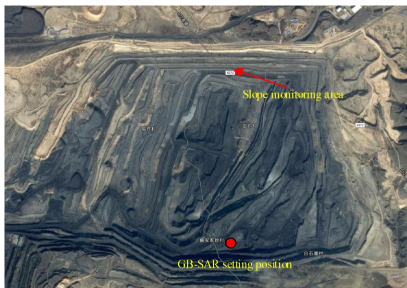
Figure 7. Ground-based interferometric radar (GB-SAR) setting position and the monitored slope.
