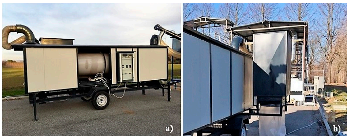
Figure 1. Rotary dryer prototype (a); dust recovery system (b).
