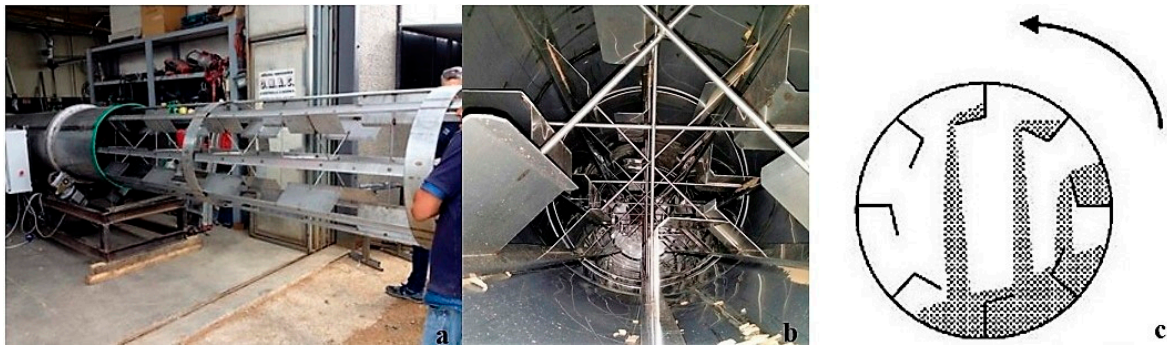
Figure 2. Intertwined flights inside of cylinder (a,b); schematic representation of the system (c).
