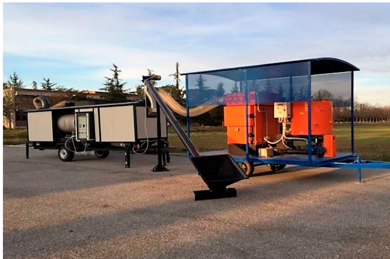
Figure 3. Mobile rotary dryer connected to a boiler of the power of 80 kW.
