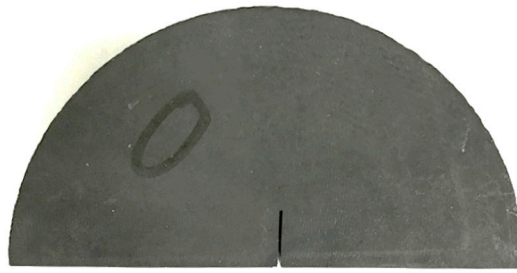
Figure 1. Notched semi-circular bend (NSCB) sample.
