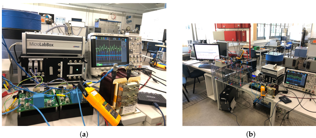
Figure 21. Experimental implementation of the three level asymmetrical topology 3L-ASYM. (a) KIT8020-CRD-8FF1217P-1 boards connected to form one leg of the 3L-ASYM converter. (b) Test bench.
