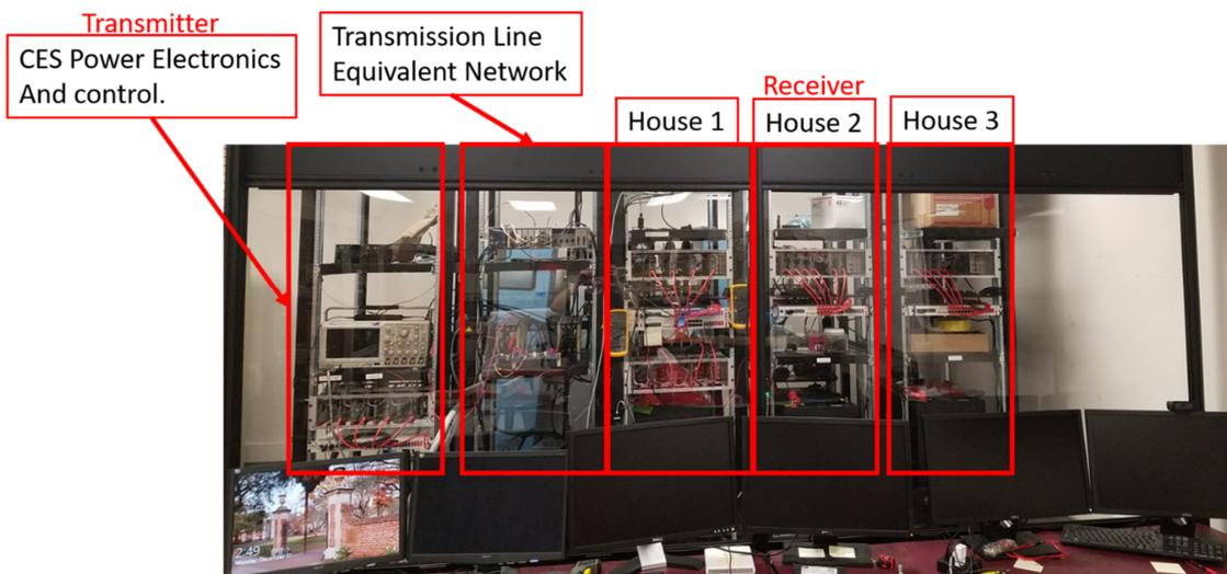
Figure 7. Live-scale DC microgrid physical setup.
