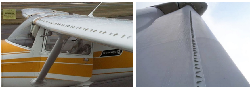
Figure 1. Applications of passive vortex generators (VGs) on the aircraft wings and wind turbine blades [15,16].
