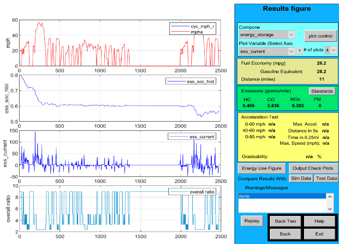
Figure 28. FTP driving speed cycle of the input HEV midsize car; HEV car speed cycle; estimated Rint Li-ion battery SOC on NREL ADVISOR- MATLAB platform, and current profile (from the top to the bottom).
