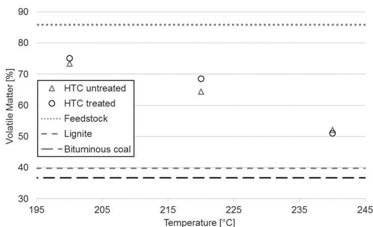
**Figure 5.** Volatile matter of hydrochar samples as a function of reaction temperature for untreated and treated wood.
