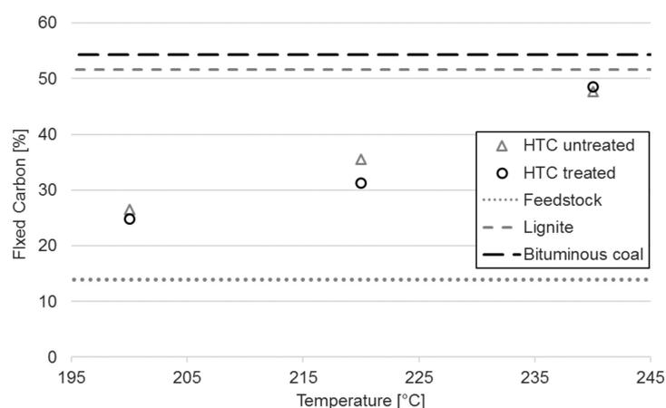
**Figure 6.** Fixed carbon of hydrochar samples as a function of reaction temperature for untreated and treated wood.
