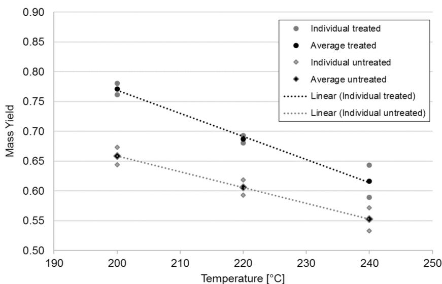
**Figure 2.** Mass yield of hydrothermal carbonization (HTC) experiments as a function of temperature for untreated and treated wood.
