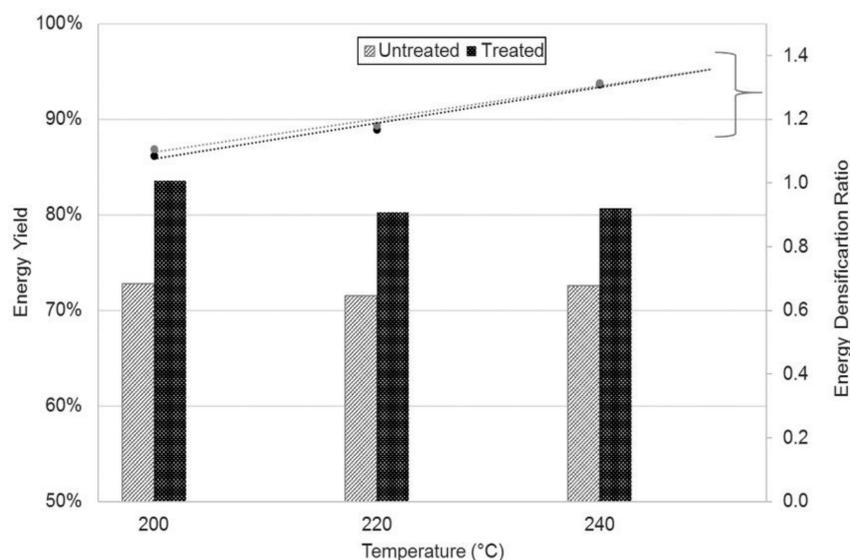
**Figure 4.** Energy yield and energy densification ratio of hydrothermal carbonization experiments as a function of reaction temperature for untreated and treated wood. Energy yield as bars is shown on left axis, while points and trendline show energy densification on right axis.
