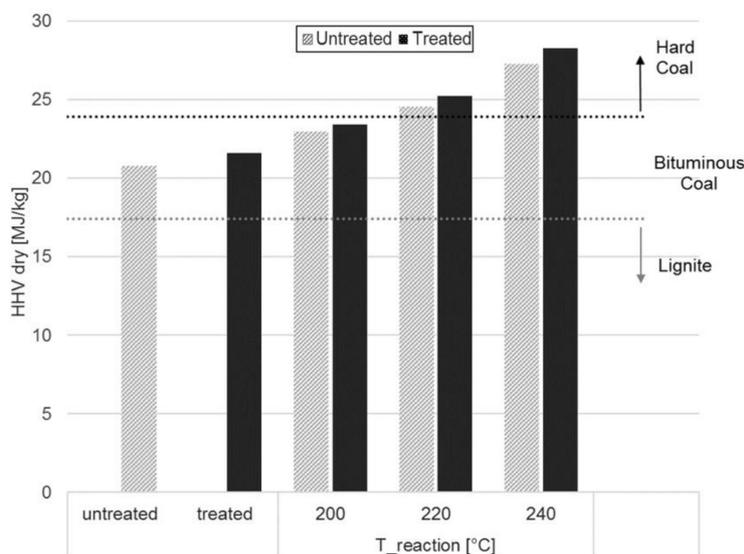
**Figure 3.** Higher heating value of hydrothermal carbonization experiments as a function of reaction temperature for untreated wood and treated wood.
