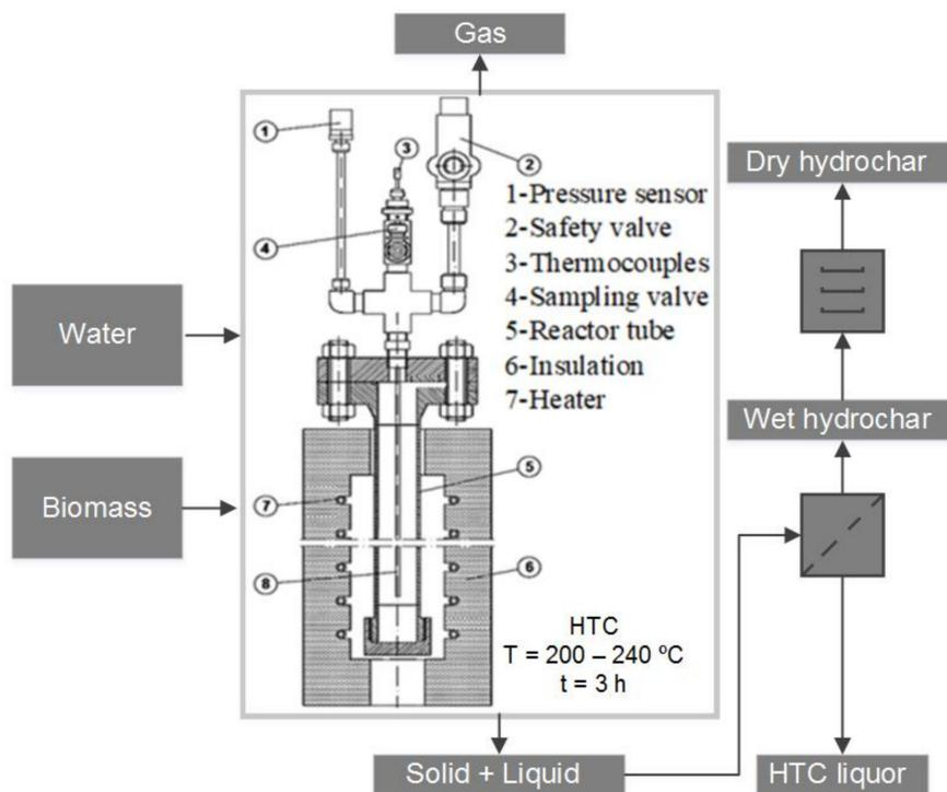
**Figure 1.** Hydrothermal carbonization (HTC) experimental unit and experimental procedure.
