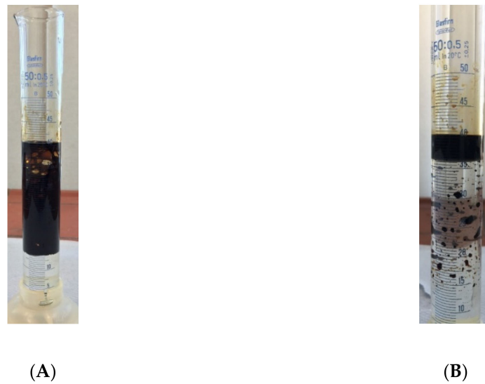
Figure 15. Oil produced after the brine flooding in the secondary mode. Phase entrapment during core flooding (A) and the same fluids after phase settlement in an oven (B).
