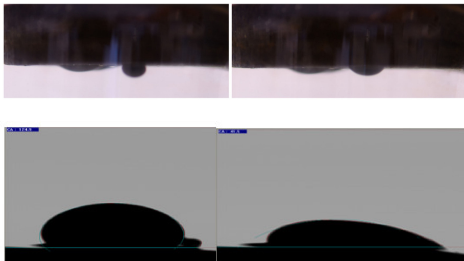
Figure 5. Contact-angle measurement between oil-saturated, six-week aged core plug and oil drop at 0 min (left side) and after 60 min (right side). Top images are obtained from in-situ device and bottom images represent the pendant drop method contact-angle measurement.
