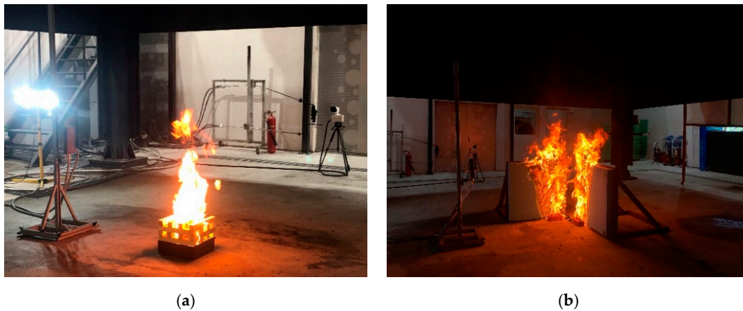
Figure 2. Independent measurement of heat release rate for (a) the wood crib and (b) polyether foam.
