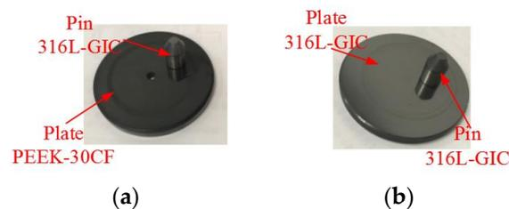
Figure 13. Two groups of matching materials for friction test: (a) 316L-GIC with PEEK-30CF; (b) 316L-GIC with 316L-GIC.
