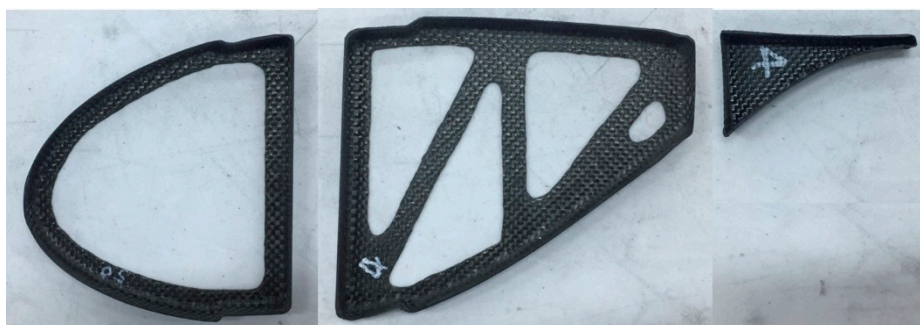
Figure 9. The truss ribs.
