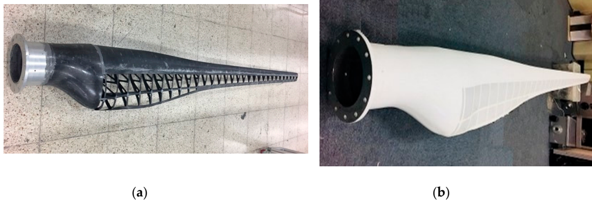
Figure 4. The fabricated fabric-covered blade: (a) without skin and (b) with skin.
