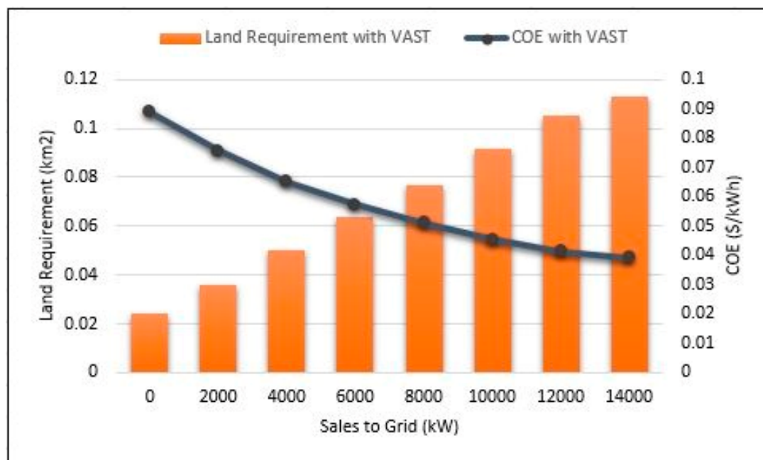
Figure 11. Land requirement and LCOE change of the system using vertical solar tracker with different sales capacity.
