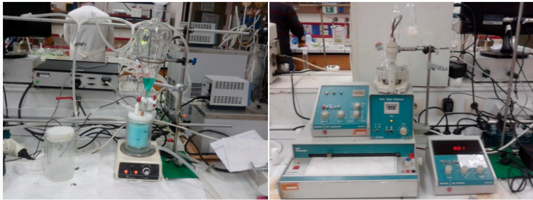
Figure S2. Presentation of the setup used for co-precipitation. (Left). The setup includes a glass funnel containing the mixed aqueous solution of \text{Ni}^{2+} , \text{Al}^{3+} and \text{Cu}^{2+} nitrates and a double-walled glass vessel, with a cover, on a magnetic stirrer that initially contained 330mL of distilled water. During the experiment, the mixed solution from the glass funnel drips at a steady rate in the glass vessel. The setup also includes a glass electrode immersed in the glass vessel and a nozzle for adding \text{NH}_4\text{OH} solution into the vessel for keeping \text{pH}=8 during co-precipitation process. (Right). A pH-control system (Mettrom) equipped with glass/saturated calomel electrode for stabilizing the \text{pH}=8 at co-precipitation vessel during catalyst preparation introducing the necessary \text{NH}_4\text{OH} solution quantities.
