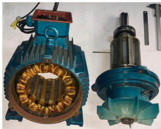
**Figure 18.** Stator and rotor of 12/8 pole SRM is shown. This SRM is a prototype.
