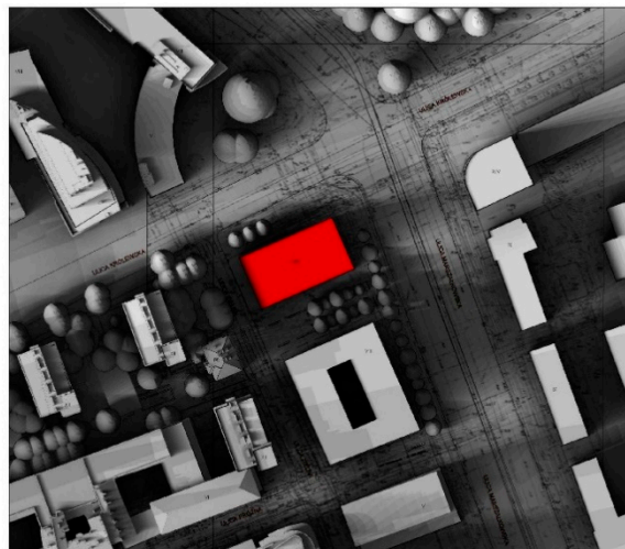
Figure 3. Summer Solstice—Collective shadow analysis for designed building.
