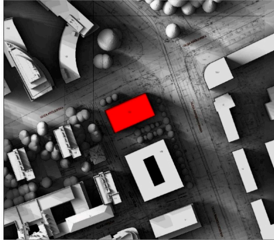
Figure 4. Spring Equinox. Collective shadow analysis for designed building.
