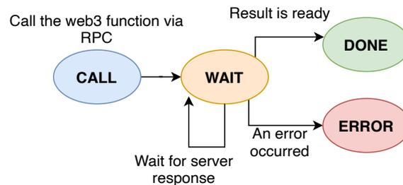
**Figure 9.** The state-transition diagram for a web3 call in the developed framework (image created using <https://draw.io>).
