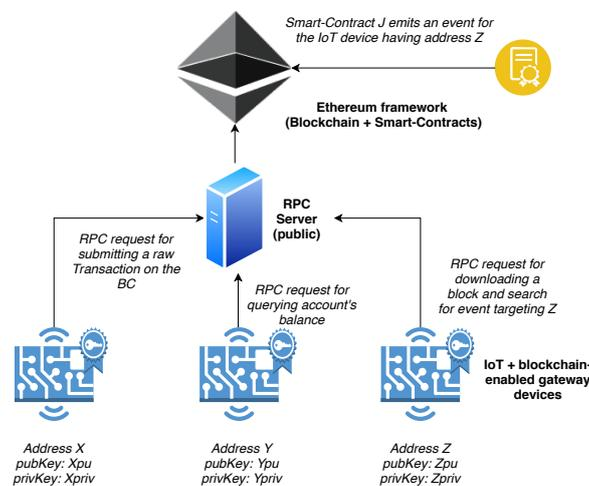
**Figure 4.** A representation of the final proposed architecture. Each IoT device has its own gateway and can sign transactions locally and offline. Each of them is also identified within the blockchain through its address and can be thus a target for possible Smart-Contract events (image created using <https://draw.io>).
