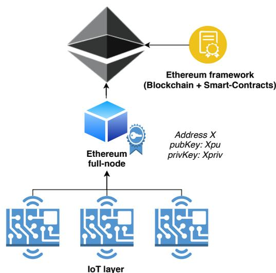
**Figure 3.** A representation of the first explored solution. IoT devices communicate with the local full node which is in charge of signing and broadcasting transactions for them. However, the IoT layer remains agnostic of the existence of the Blockchain. It simply sends data to a local centralized entity (image created using <https://draw.io>).
