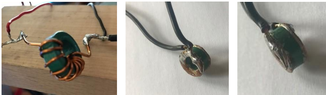
Figure 5. Tested inductors containing toroidal cores.
