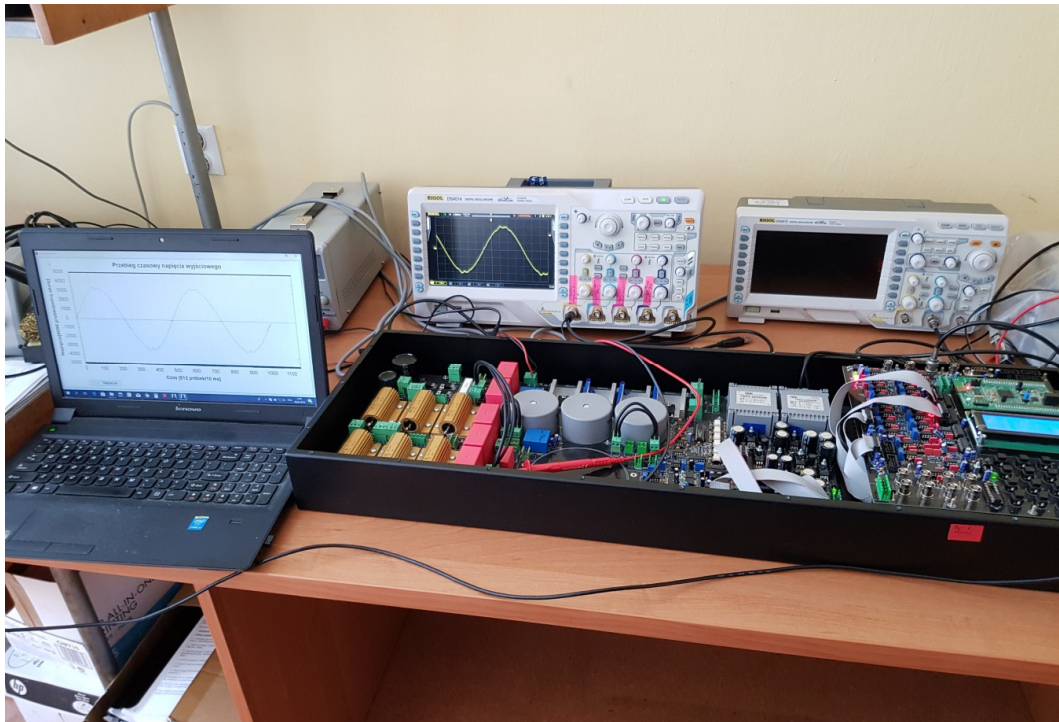
Figure 11. The experimental VSI model and PC with dedicated visualization software.
