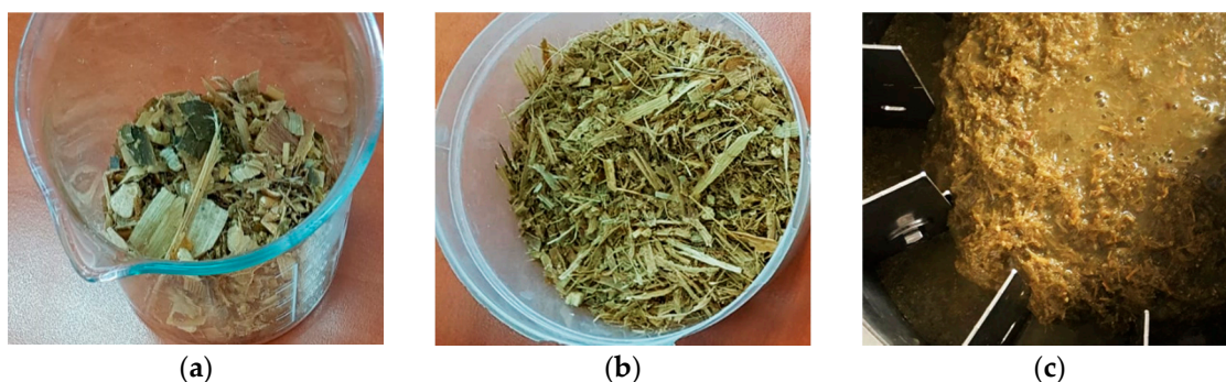
Figure 4. Maize silage: (a) Raw maize silage; (b) shredded maize silage; and (c) hydrated maize silage used in the hydrodynamic disintegration process.
