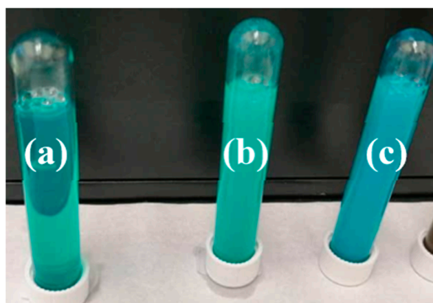
Figure 10. Gel formed by CuAc at room temperature at various pH values: (a) No gel at pH = 5.23 and weak gel at (b) pH = 7 and (c) pH = 11.
