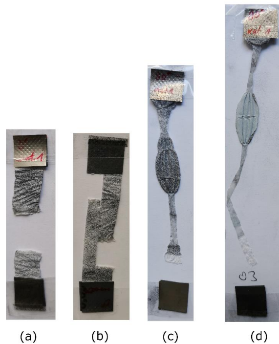
Figure 5. Examples of extreme behavior: (a) relatively brittle fracture in the center, representing the desired, best behavior; (b) failure along the specimen length; (c) intermediate stabilization and localization in different areas; (d) extreme elongation with two different localization areas in the specimen.
