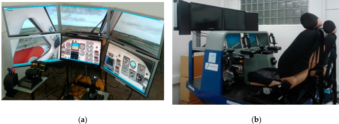
Figure 2. The flight simulators in use—(a) the fixed-base flight simulator and (b) the moving-base flight simulator.
