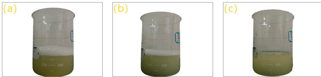
Figure 6. The basic fluid is added with 0.10% (a) TX-10, (b) HSB1618 and (c) penetrant T.
