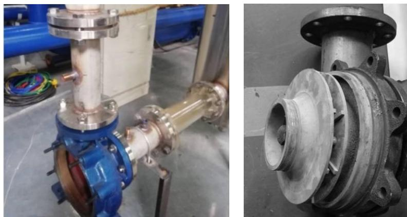
Figure 5. TBD pump casing (left) and impeller (right).
