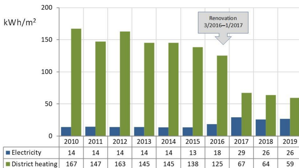
Figure 6. Annual specific district heat and electricity consumption. The renovation was done from March 2016 to January 2017.
