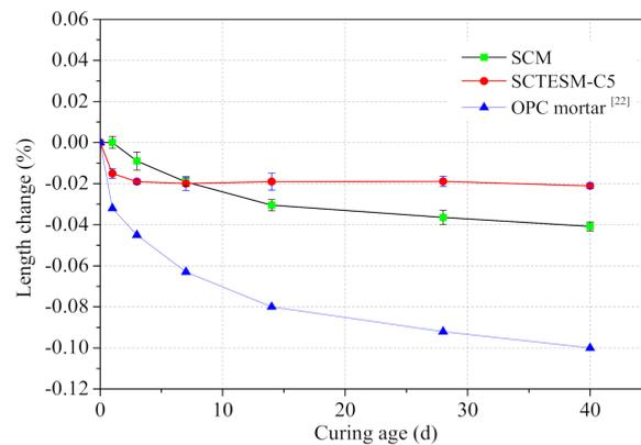
**Figure 12.** Comparison of volume shrinkage between SCM and SCTESM-C5.
