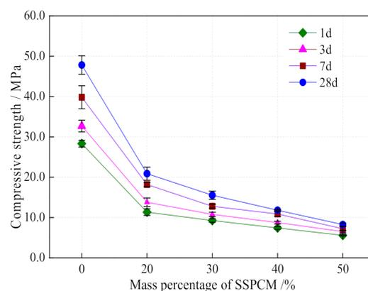
**Figure 16.** Compressive strength of SCTESM.
