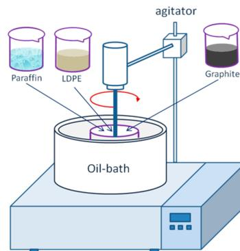
**Figure 3.** Schematic of shape-stabilized phase change material (SSPCM) preparation.
