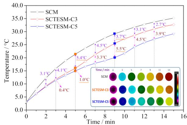
Figure 14. Upper surface temperature and infrared thermography images.
