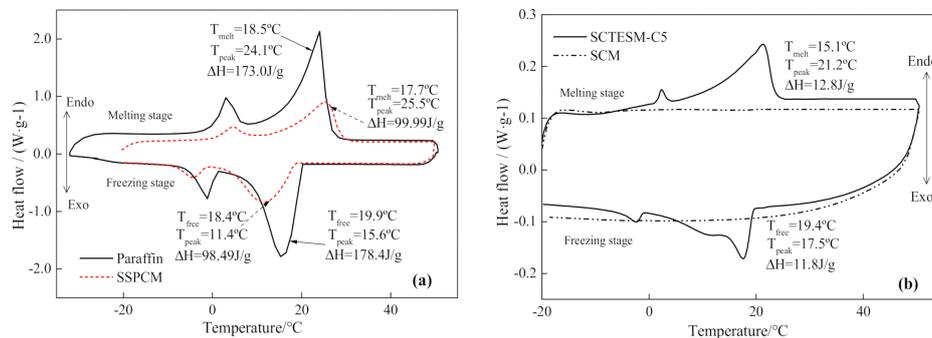
**Figure 9.** Differential scanning calorimeter (DSC) curves: (a) paraffin and SSPCM; (b) SCTESM-C5 and SCM.
