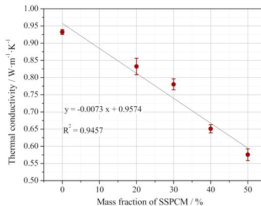
**Figure 11.** Thermal conductivity change of SCTESM with different dosages of SSPCM.
