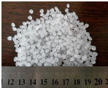
Figure 1. Low density polyethylene (LDPE).
