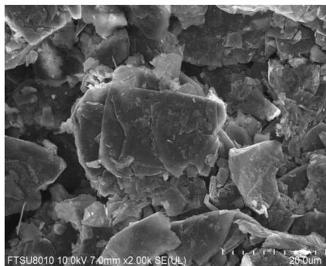
Figure 2. SEM image of flake graphite.
