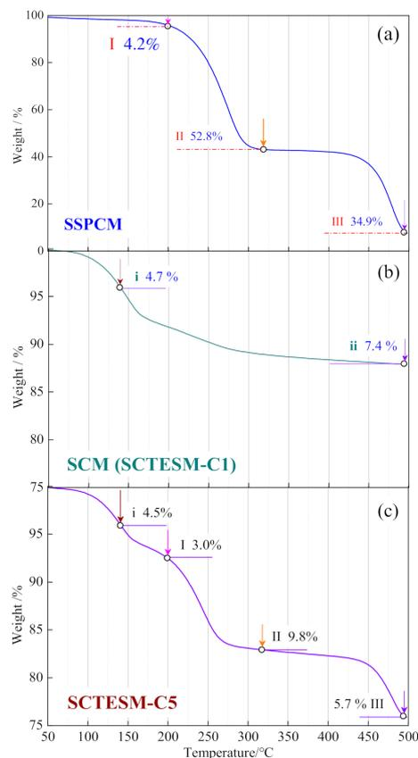
**Figure 10.** Thermogravimetric analysis curves: (a) SSPCM; (b) SCM; (c) SCTESM.
