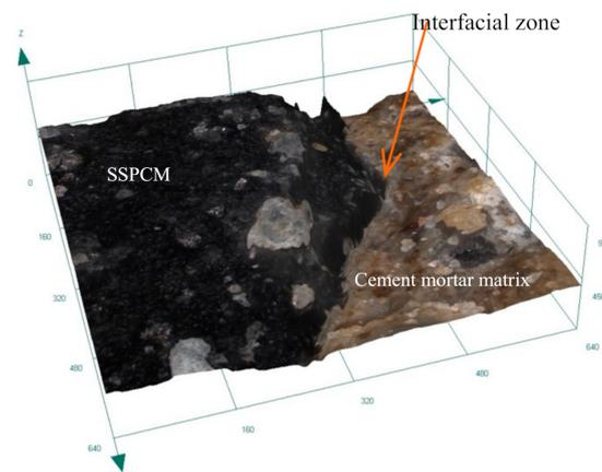
**Figure 13.** LSCM image of interfacial transition zone of SCTESM.
