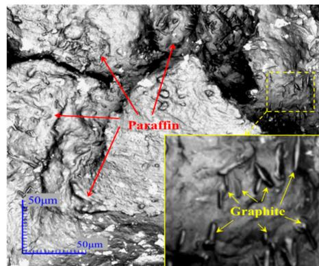
**Figure 6.** Laser confocal scanning microscope (LSCM) image of graphite distributed in SSPCM.
