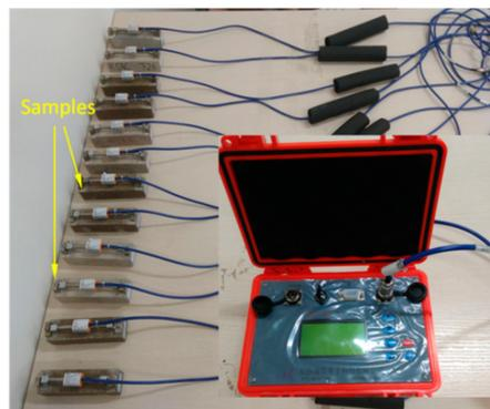
**Figure 7.** Device of length change test system.
