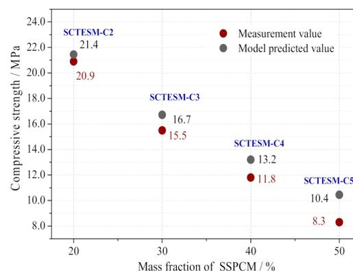
Figure 18. Compressive strength measurements versus model predicted values.
