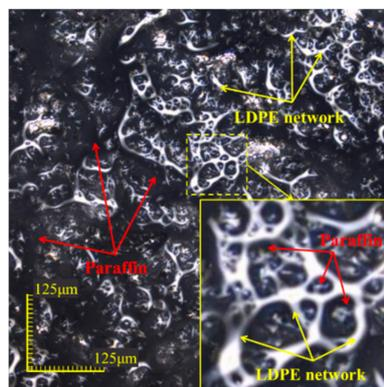
**Figure 5.** LCSM image of SSPCM network structure.
