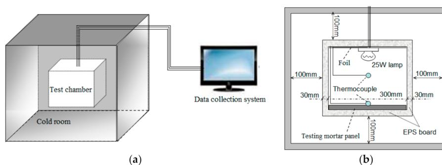
**Figure 8.** Schematic of the experimental device: (a) overall schematic, (b) cross-sectional view.
