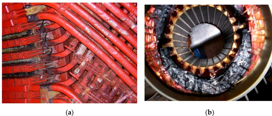
**Figure 2.** Stator winding faults: (a) short circuit in a high voltage winding; (b) short circuit in a low voltage winding.
