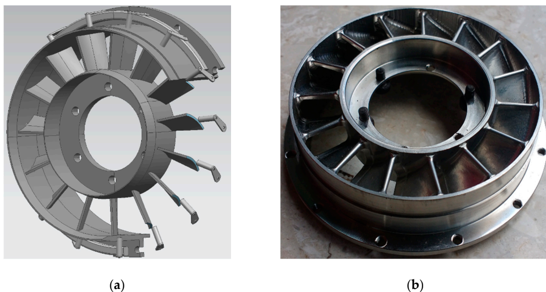
Figure 4. Researched adjustable turbine nozzle system: (a) 3D model of the variable geometry system; (b) manufactured nozzle with modified geometry (nozzle angle inclination increased +5^\circ ).
