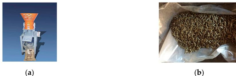
**Figure 3.** N-Pico pelletizer (a) and pelletized rice straw (RS) (b).
