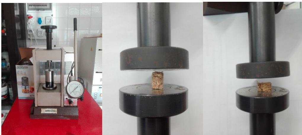
Figure 4. Axial compressive test.
