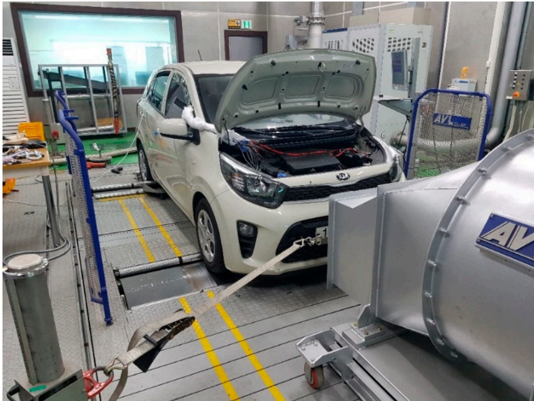
Figure 8. Test on the chassis dynamometer for verification. By comparing the experimental and simulation results the feasibility of the modeling method can be determined.
