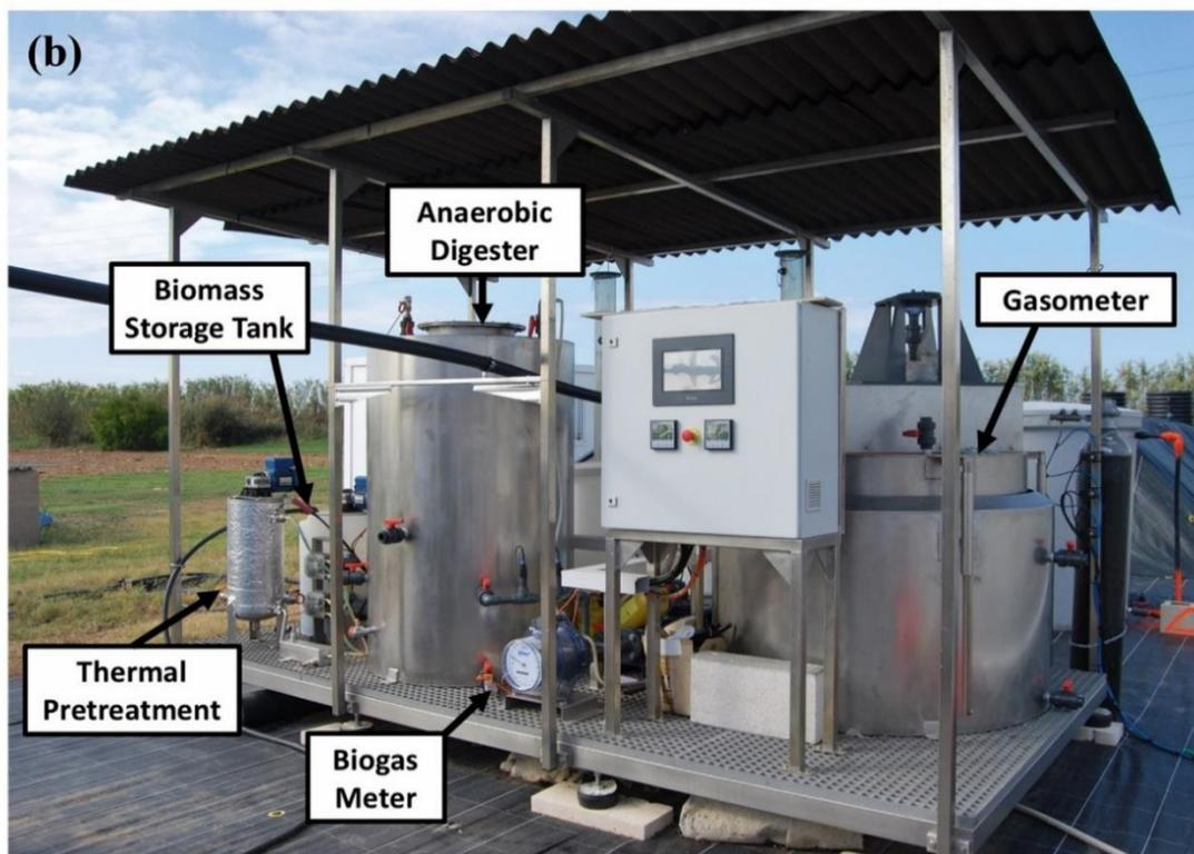
**Figure 2.** (a) Diagram of the anaerobic digestion plant. Mixers (M), pumps (P), electrical resistances (ER) and electrovalves (EV) are indicated in the figure, as well as the temperature (T), liquid level (LI), pressure (PI), redox and pH sensors. (b) Image of the anaerobic digestion plant.
