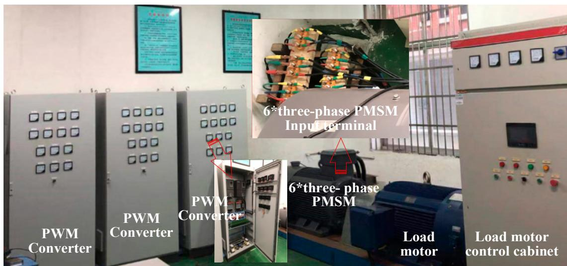
Figure 22. 6\*three-phase PMSM experimental platform.
